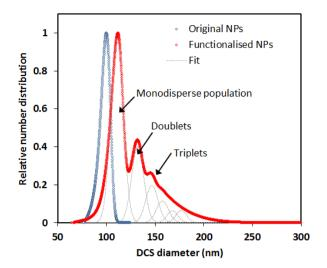
CPS size distribution of polystyrene nanoparticles (NPs, blue  $\diamond$ ) and the same NPs functionalised with Immunoglobulin G (IgG) antibodies (red  $\diamond$ ). The high resolution size distribution of the functionalised particles allows identification and quantification of monodisperse NPs and those agglomerated in doublets, triples or larger aggregates.
