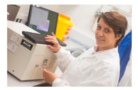
Dr Caterina Minelli of the NPL's Nanoanalysis Group using the CPS Disc Centrifuge technique for nanoparticle size and density characterisation.
